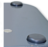
Dual antenna RTK-GPS for accurate localization
